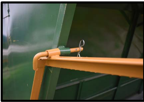
J-Pin Locked in Feeding Position
