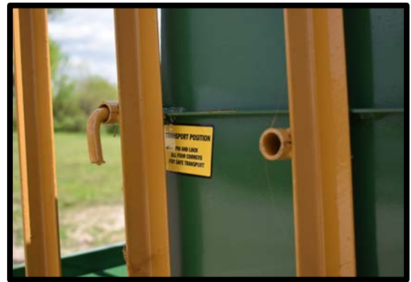
J-Pin Locked in Transport Position
